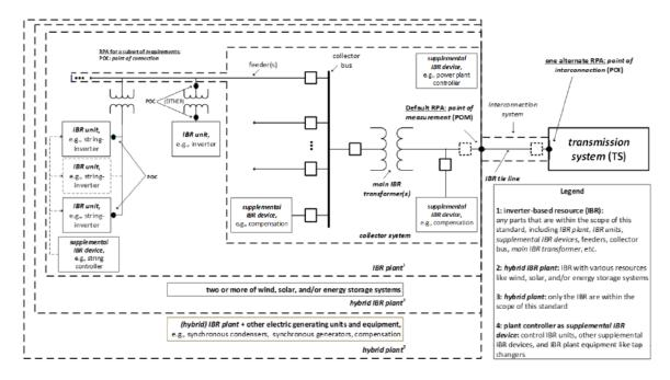
NOTE 1—The POM is the default RPA. Moving the RPA from the POM to the POI may exceed the technical minimum requirements specified in this standard and may require deliberate consideration of the pros and cons. For example, the ability of *IBR plants* to meet the performance requirements in this standard may be impacted if the *IBR owner* is not allowed to install their measurement and control equipment at the POI substation.<sup>21</sup>
